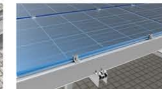
Fix panel and rail with mid/end clamps.
