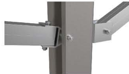
③ Post with bracing support details
