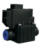
Water purifier pressure switch DNT-PS series pressure switches which we named as HP001 high pressure switch and LP001 low pressure switch are mainly designed for protection of water purifier. HP001 is a high pressure switch which will cut off the circuit when the pressure in the water tank reach to switch setting point in order to stop the RO pump working.
